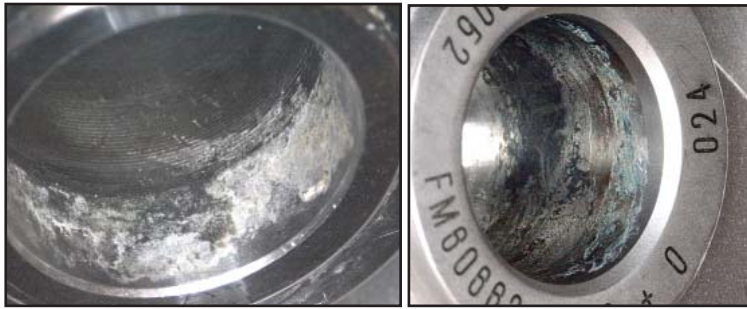
Fig 5. Examples of crevice corrosion and fretting
