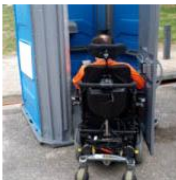
Figure 1: Picture showing accessible temporary toilet style A not meeting the needs of a wheelchair bound patron (Bromley, 2014).
