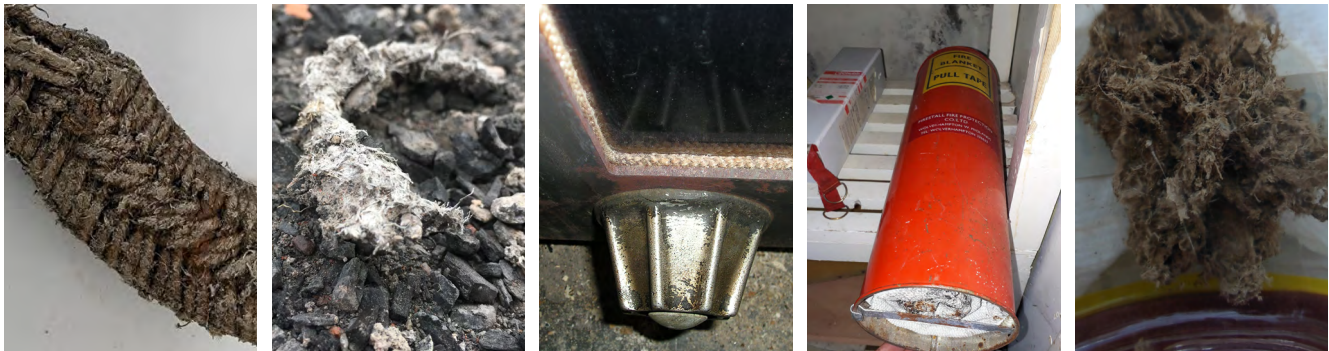
Figure 6 Examples of known asbestos-containing materials – fibre rope seal, textile materials and weathered low density fibre board.
