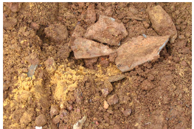
Figure 1 Asbestos cement fragments in soil.
