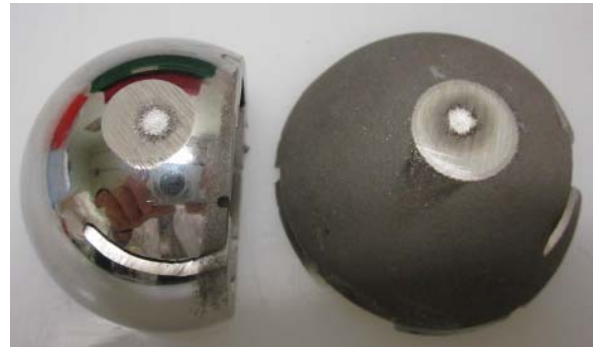
MoM components after spark tests
